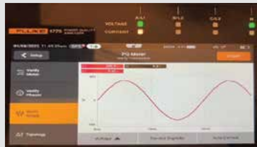
Power waveform of PFC-iPL303 during peak processing
